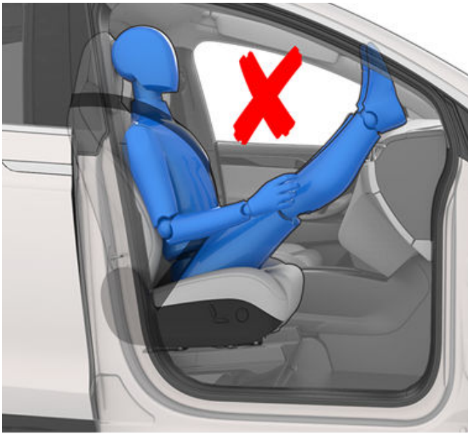
Incorrect seating position - the passenger must not slide forward on the seat cushion:
