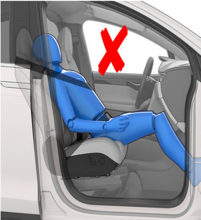
Incorrect seating position - the passenger must not recline the backrest to a laying down position when the vehicle is moving:
