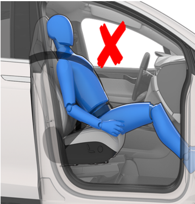
Incorrect seating position - the passenger must not recline the backrest to a laying down position when the vehicle is moving:
