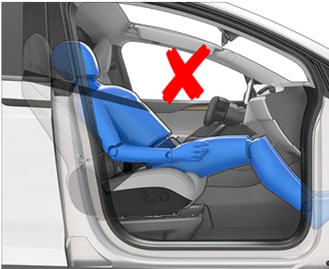
Incorrect seating position - the passenger must not recline the backrest to a laying down position when the vehicle is moving:
