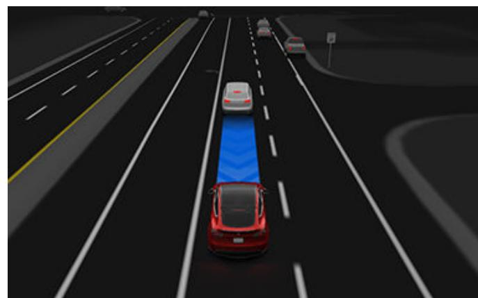
The visualization will also inform you of the system's intended action by displaying a message on the 觸控式螢幕, such as when the vehicle is slowly creeping for visibility to take a turn at an intersection.
