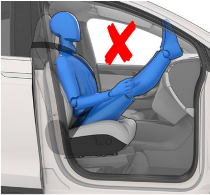
Incorrect seating position - the passenger must not slide forward on the seat cushion:
