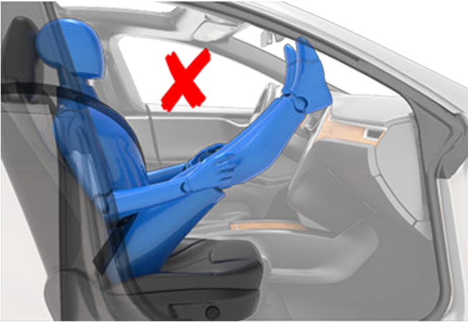
Incorrect seating position - the passenger must not slide forward on the seat cushion:
