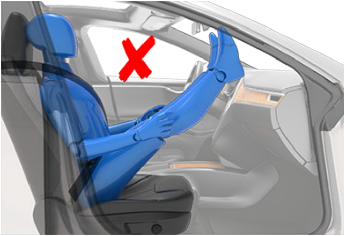
Incorrect seating position - the passenger must not slide forward on the seat cushion:
